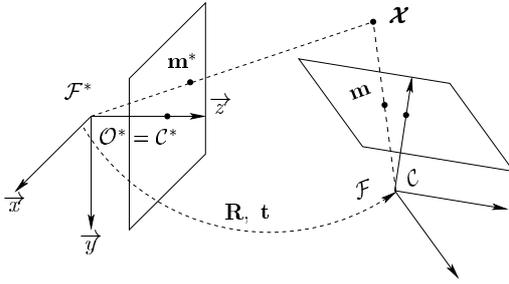
Figure 1. Perspective projections of a 3D point
