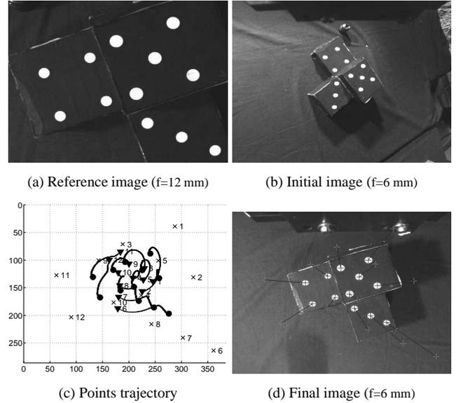
**Figure 4. Vision-based control using a 12mm lens for learning and a 6mm lens for servoing.**
