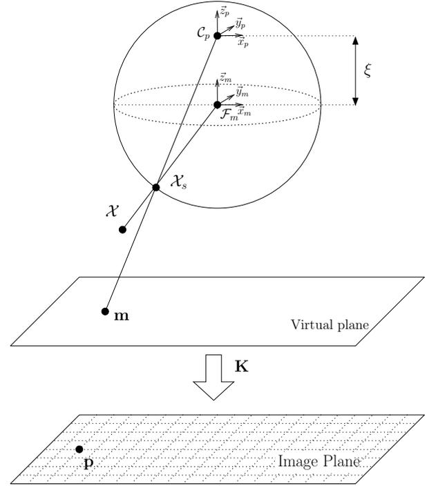
Fig. 1. Projection model for central catadioptric cameras
