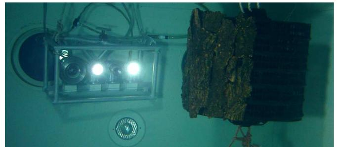
Fig. 9. In pool trials with the stereovision system and a 3D target
