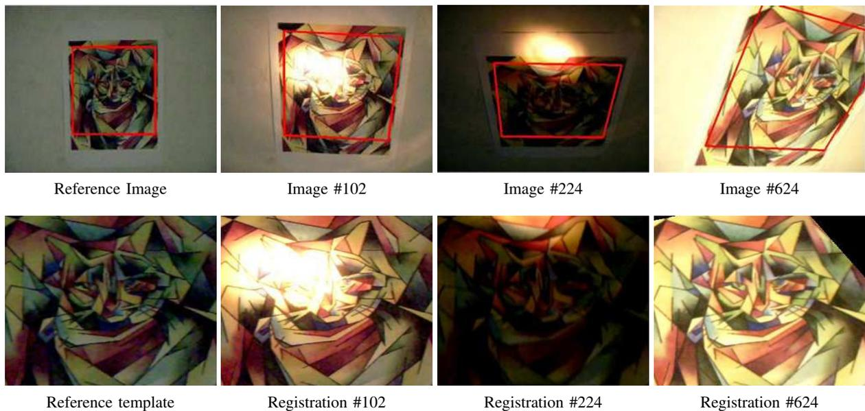
Fig. 2. (First row) Image registration of a reference image (the first one) to successive frames of a video sequence. (Bottom row) Aligned (warped) images are shown to demonstrate the stability of the tracker. The sequence contains severe changes in the specular, diffuse and ambient reflections.
