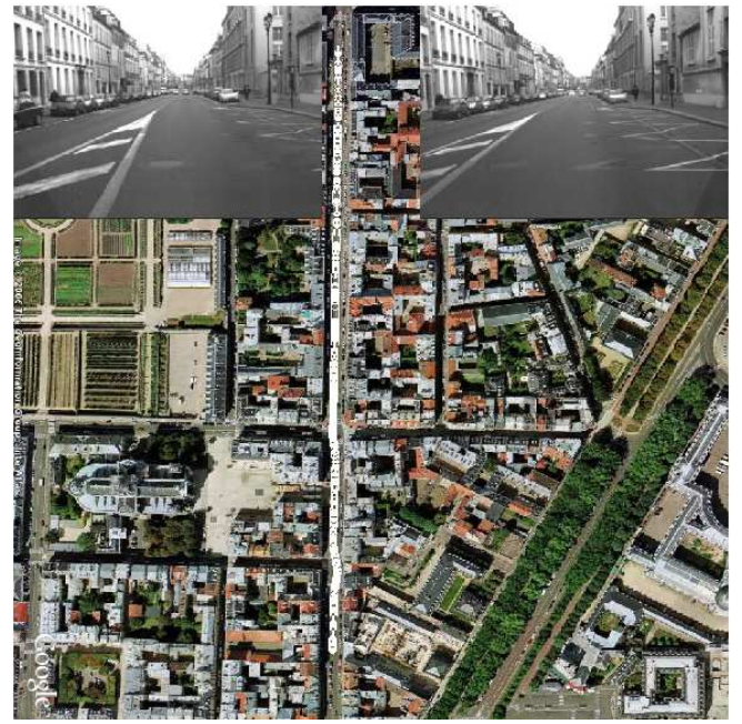
Fig. 5. Trajectory tracking around along a road in Versailles : (a) The trajectory shown in white has been superimposed on a satellite image. An typical stereo image is shown at the top.
