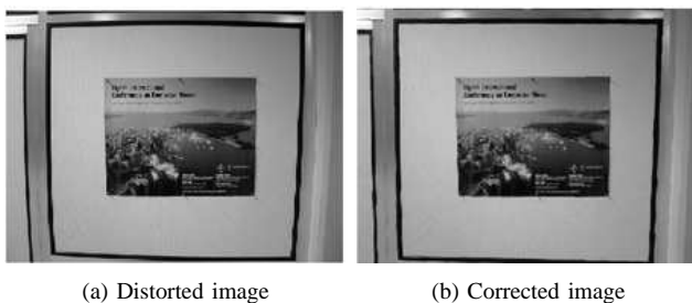
Fig. 7. Correction of the radial distortion using unstructured images and verification using a structured image with straight lines.
