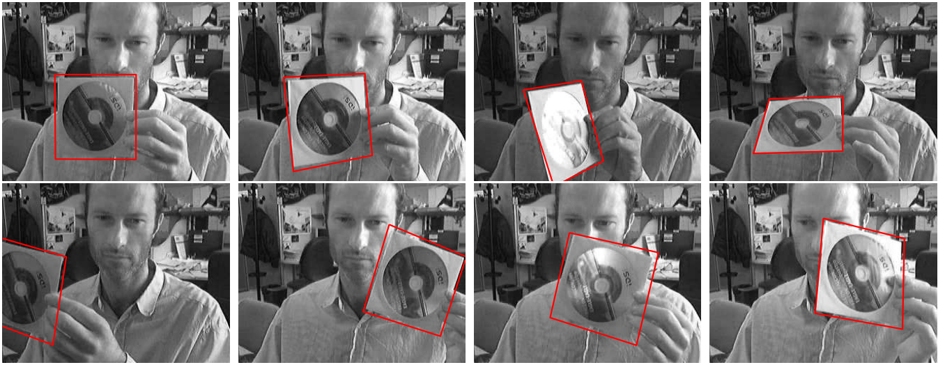
Fig. 8. Robust visual tracking of a planar target with the ESM algorithm. The output of the algorithm is a homography matrix.
